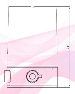
SUITABLE FOR BULLET CAMERA INNER DEPTH 150/200MM
